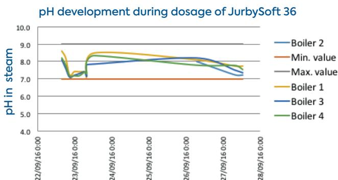
Finally, boilers 1 and 2 went for repairs. During the repairs in boilers 1 and 2, the baffle plates of the separation system and the partitions between the salt and clean compartment in the upper drums were repaired. These efforts resulted in positive outcomes. No difference in pH readings was observed in all boilers with the dosage of product 30–35 g/m<sup>3</sup> of steam (see graph below).
